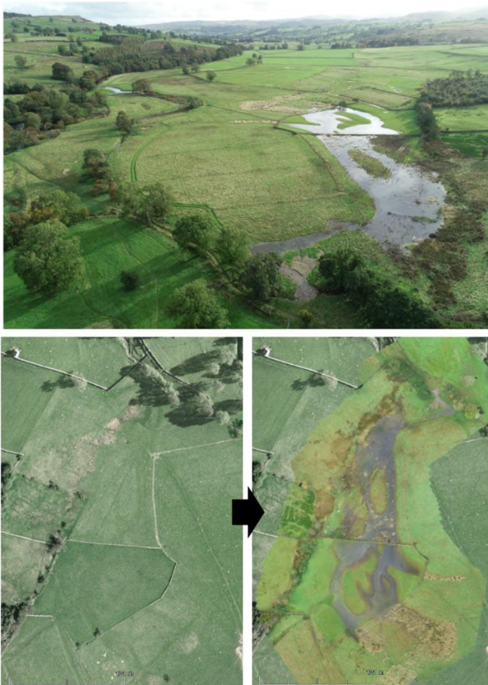
Figure 3.3 Example large wetland area created by through tributary blocking of Milkeld Sike on the Lowther Estate. Indicative of possible winter / rainstorm wetting of the North Brook site.
