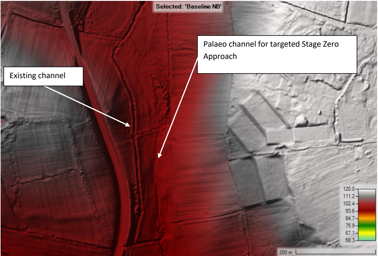
Figure 2.2 LIDAR and profile across study reach showing potential high-level opportunities and palaeo channel across the floodplain
